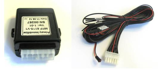
This is an independent unit that performs physical disconnection of the vehicle circuit by means of an electrical relay. The Cello-AR Security system provides two kinds of smart immobilizer; wire and wireless. All smart immobilizers are managed through the keypad via SNet communication. The wired AR Immobilizer is provided with a dedicated harness including status led.
