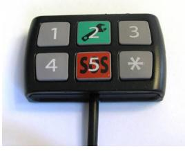
The AR keypad is the interface of the system. It is used to control the system and manage system states, including driver authentication, password changes, Ecall, BCall and any operation which requires driver or technician inputs.
